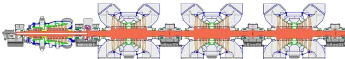
**Fig. 13 HPC longitudinal cross sections of the turbine K-800-130/3000**
