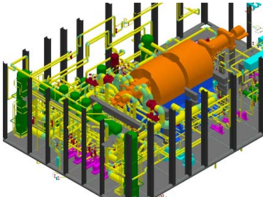
**Fig.11 Overview of the half-speed turbine plant lay-out model
