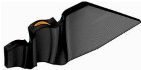
9a. Calculation grid of LPC two last stages made in AUTOGRID 5
