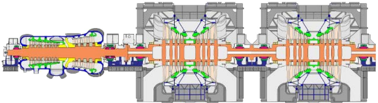
**Fig. 8 Low-speed turbine for VVER TOI project**
