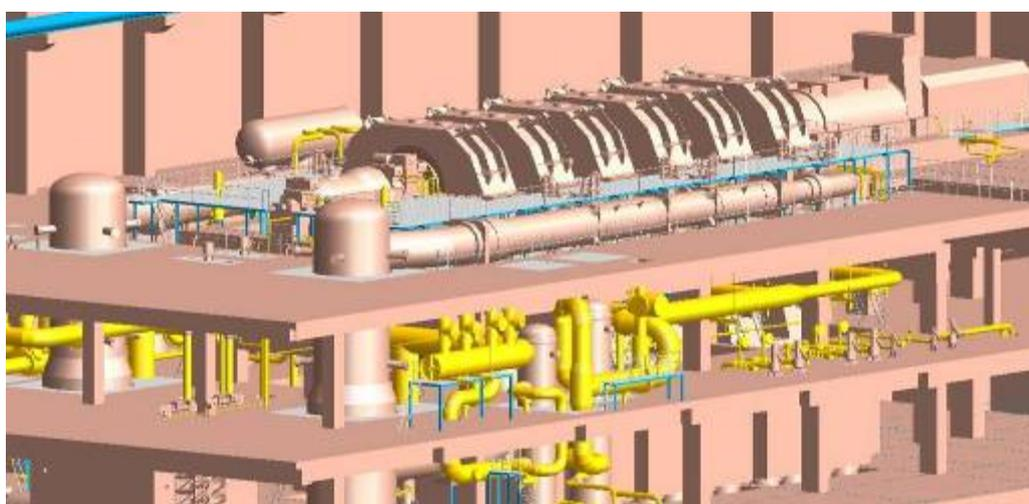
**Fig. 14 K-800-130/3000 turbine plant equipment lay-out in the turbine hall of the Beloyarskaya NPP, Russia**
