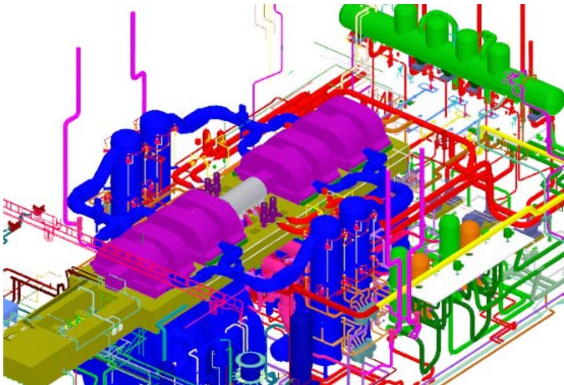
**Fig. 5 Arrangement of the turbine plant K-1200-68/3000 equipment in the turbine hall of Leningradskaya NPP-2, Russia**
