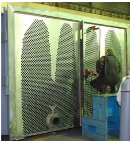
**Fig. 15. Block-modular construction of the 1000MW turbine condenser at Kozloduy NPP**
