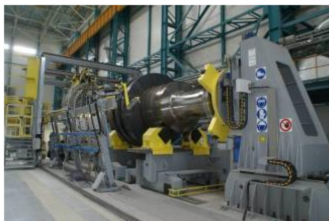
Spanning type welding skid for the rotors horizontal welding
