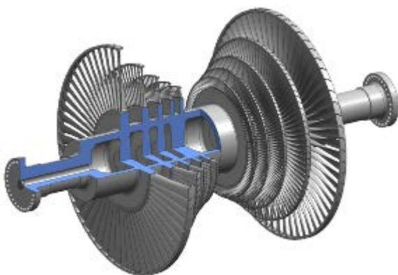
Low pressure rotor of the half-speed turbine
