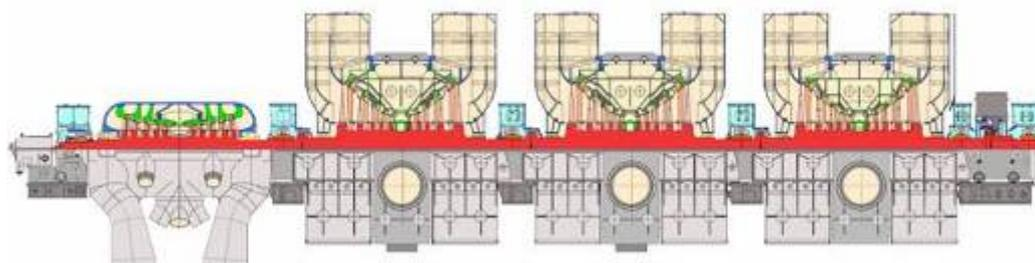
**Fig. 2 Steam turbine K-1000-60/3000-3 for Bushehr NPP in Iran**
